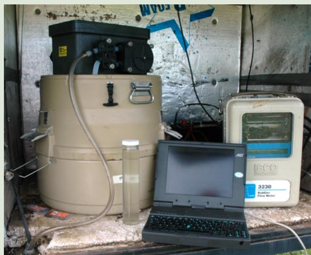
Automated water monitoring equipment used in ISA watershed programs collects and stores data that can be transmitted electronically. Photos: Keegan Kult
